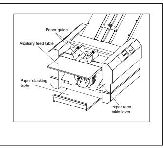
\* Place the paper with its printed side down in case of fold-out.
